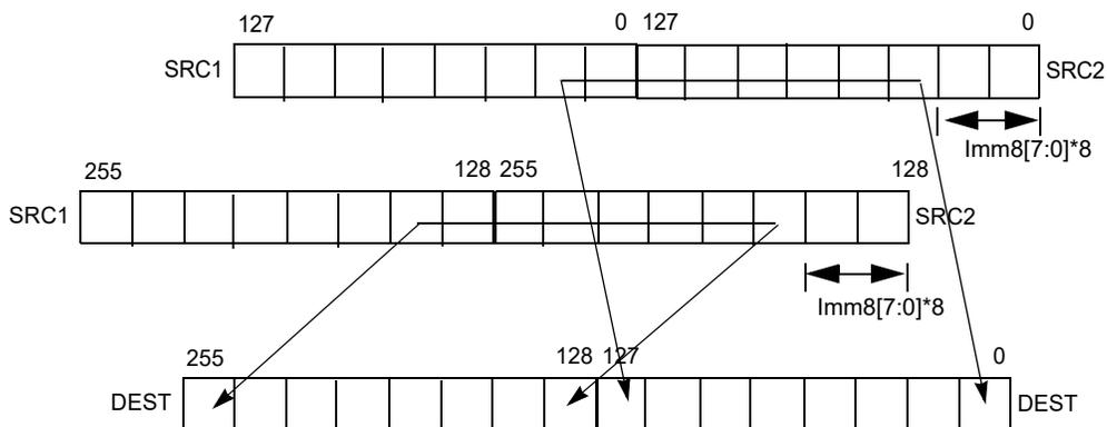
Figure 4-7. 256-bit VPALIGN Instruction Operation
