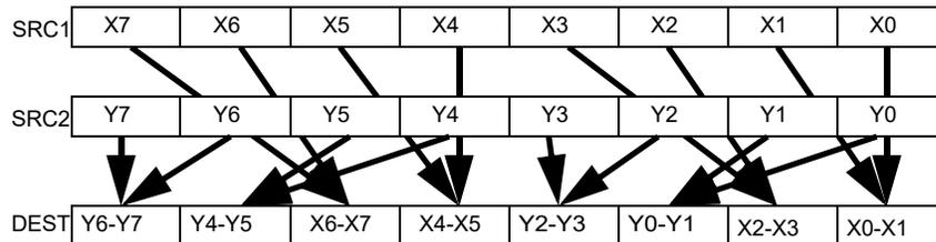
**Figure 3-23. VHSUBPS operation**
