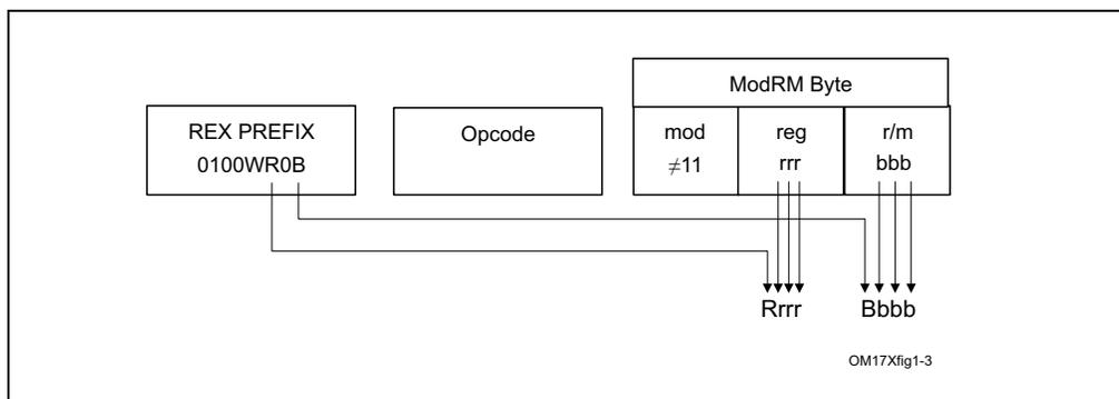
**Figure 2-4. Memory Addressing Without a SIB Byte; REX.X Not Used**
