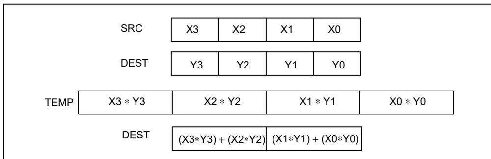
Figure 4-11. PMADDWD Execution Model Using 64-bit Operands
