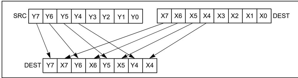
**Figure 4-20. PUNPCKHBW Instruction Operation Using 64-bit Operands**
