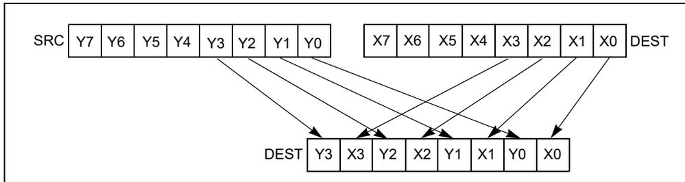
Figure 4-22. PUNPCKLBW Instruction Operation Using 64-bit Operands
