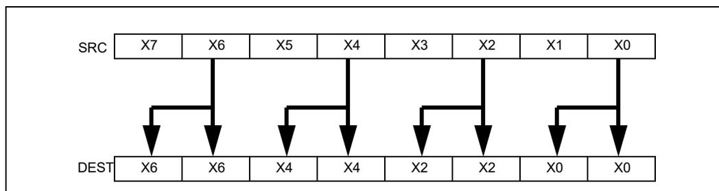
Figure 4-4. MOVSLDUP Operation
