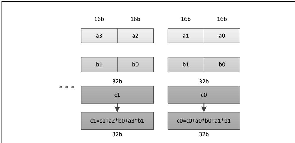
Figure 7-1. Register Source-Block Dot Product of Two Signed Word Operands with Doubleword Accumulation<sup>1</sup>
