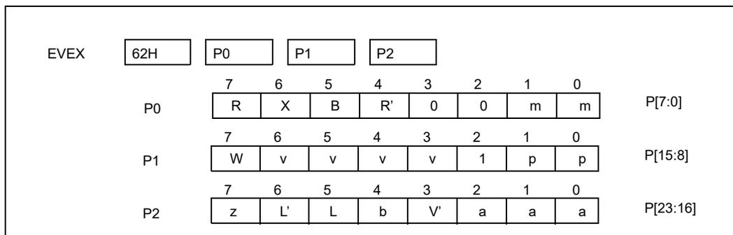
Figure 2-11. Bit Field Layout of the EVEX Prefix<sup>1</sup>
