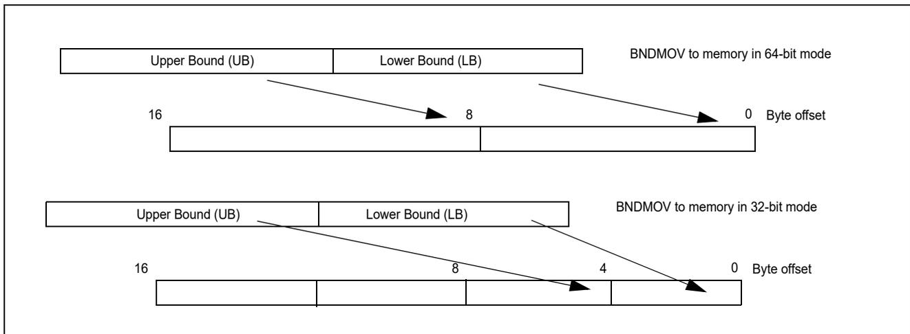
Figure 3-5. Memory Layout of BNDMOV to/from Memory
