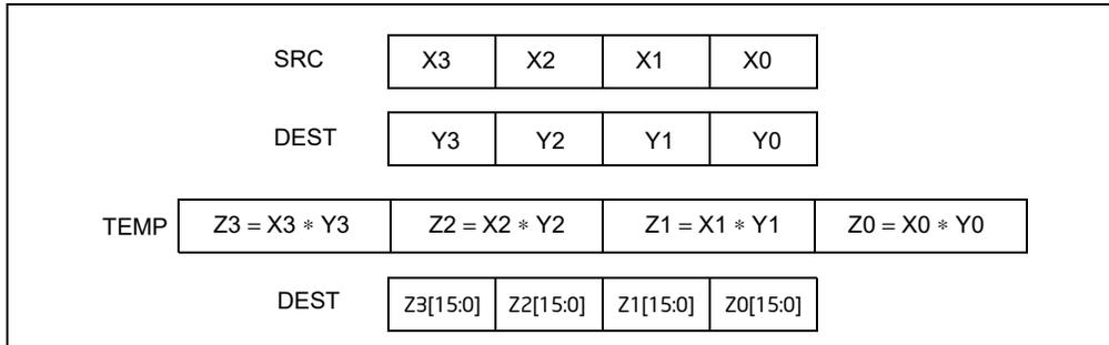
Figure 4-13. PMULLU Instruction Operation Using 64-bit Operands
