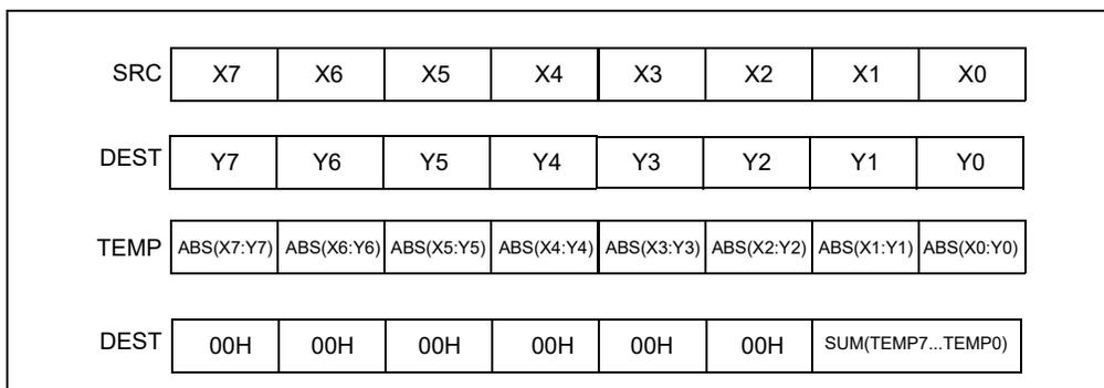
**Figure 4-14. PSADBW Instruction Operation Using 64-bit Operands**
